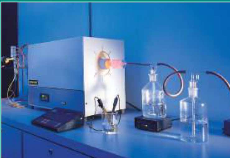
Halogen Content & Corrosivity Tests Equipment - IEC 60754-1 & IEC 60754-2
