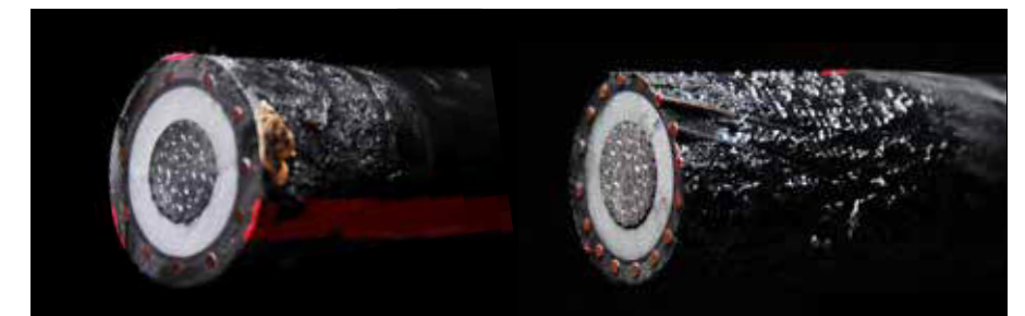
Cable Protected with Scotch® Fire Retardant Electric Arc Proofing Tape 77 after test
