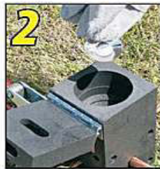
2 Place metal disc in bottom of mold crucible.
