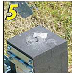
5 Ignite the starting powder with the Flint Ignitor.
